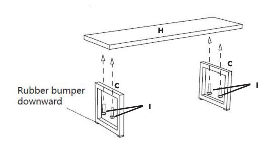
3b. Using M8\*45 screws, tighten mini-shelf frame pieces to the shelf top. NOTE: This pieces does NOT attach to the display table. It will rest on top of the unit.
