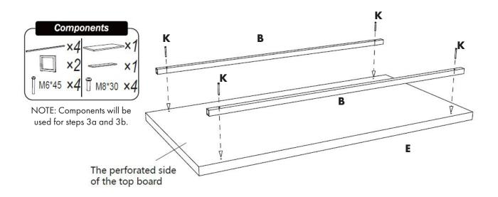
3a. Flip tabletop over, then secure support rods to its underside using M6\*30 screws. (Underside is perforated with pre-drilled holes.)
